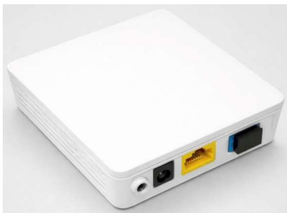
Fig. 4. ONU subscriber terminal (P=5W) for connecting the subscriber to the GPON network.
