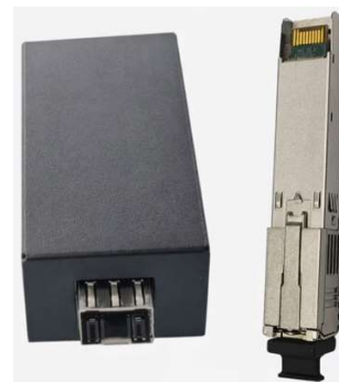
Fig. 2. Mini OLT GPON equipment for SOHO network deployment: (a) compact media converter ( P=18W ) with LC duplex optical connector for connection to PLC splitter 1:32; (b) GPON SFP OLT transceiver (Class B+, downstream 2.488 Gbps at \lambda=1490 nm, upstream 1.244 Gbps at \lambda=1310 nm)
