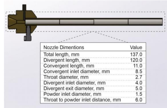
Fig. 1. Schematic views with dimensions of the low-pressure cold spray nozzle
