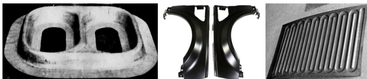
Fig. 7. Typical panels of transport equipment. Overall dimensions: 350x600...800 mm. Materials – alloys of Al, Mg, Ti, Nb
