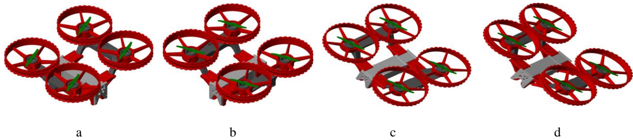
Fig. 7. Visual orientation of the physical quadrotor model at key simulation milestones: a – prior to yaw rotation (5 s); b – post-yaw rotation and prior to roll maneuver (10 s); c – during roll rotation and prior to pitch maneuver (11 s); d – post-pitch rotation (15 s)
