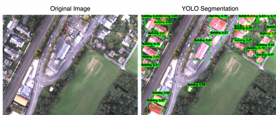
Fig. 5. An example of building segmentation on an image from the VPAIR dataset [21]
