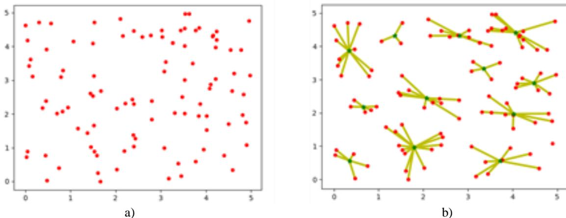
Fig. 5. The process of algorithm functioning to determine the initial centroids using Small Step algorithm: a) a set of points (consumers), b) defining the centroids
