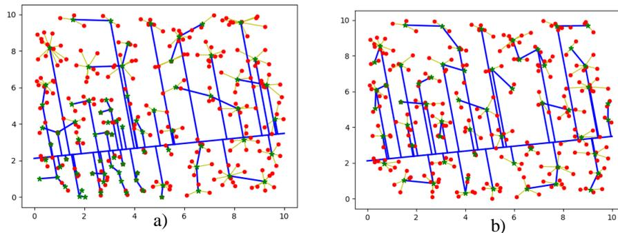
Fig. 6. Examples of distribution grid topologies: a) topology example with the estimated cost  $C = 943201.31$  USD, b) topology example with the estimated cost  $C = 722356.66$  USD
