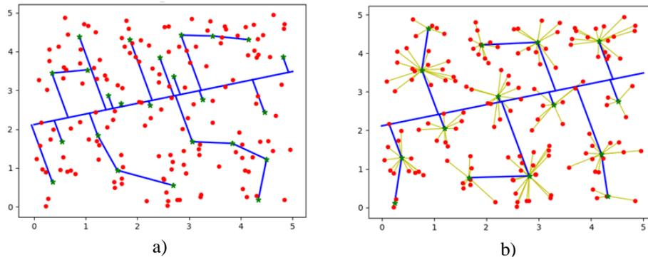
Fig. 7. Example EPS distribution grid: a) existing EPS distribution grid, b) results of EPS distribution grid reengineering
