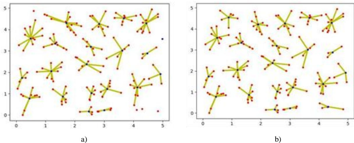
Fig. 2. Comparison of classical k-means (a) algorithm and its modifications with connection length restriction (b)
