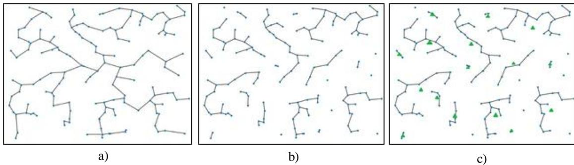
Fig. 4. The process of algorithm functioning to determine the initial centroids using minimum spanning tree creation (Prim's and Kruskal's algorithm) a) creation of a minimum spanning tree, b) elimination of edges failing to meet the condition, c) definition of centres
