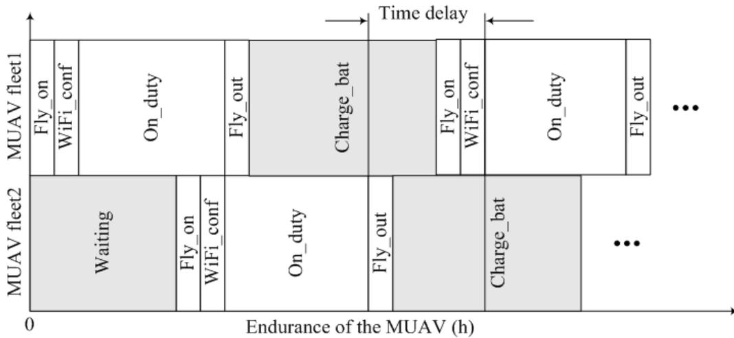
Fig. 2. Shift schedule for 2 MUAV fleets with time delay
