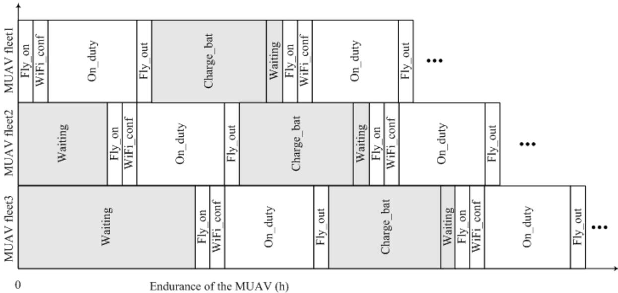
Fig. 3. Shift schedule for 3 MUAV fleets ensuring the persistent operation of the UEWN for ZNPP monitoring missions
