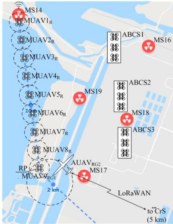
Fig. 1. Scheme of deployment of a UEWN used for Zaporizhzhia NPP monitoring (ZNPP) to connect MS14 with the CrS in case of damage of the wired network between MS14 and the CrS
