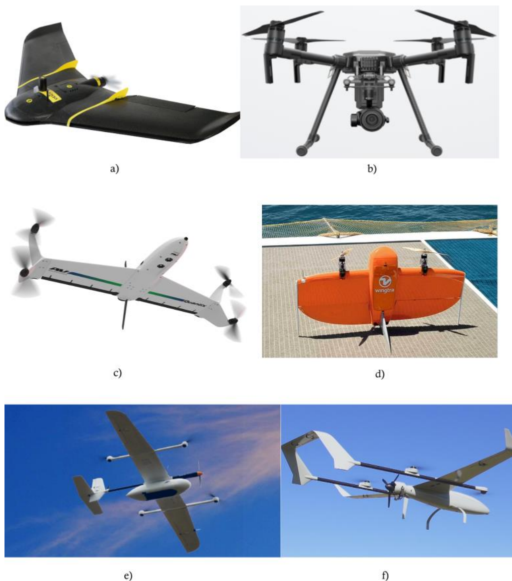
Fig. 6. Unmanned Aircraft Vehicles for photogrammetric purposes: a) Fixed-wing Ebee SenseFly [11], b) Multirotor Matrice 200 DJI [12], c) VTOL Tail seater Quantix AeroVironment [13], d) VTOL Tail seater Wingtra [14], e) VTOL Simplistic Configuration CW-10 JOUAV [15], f) VTOL Simplistic Configuration Transi-tion Alti UAS [16]
