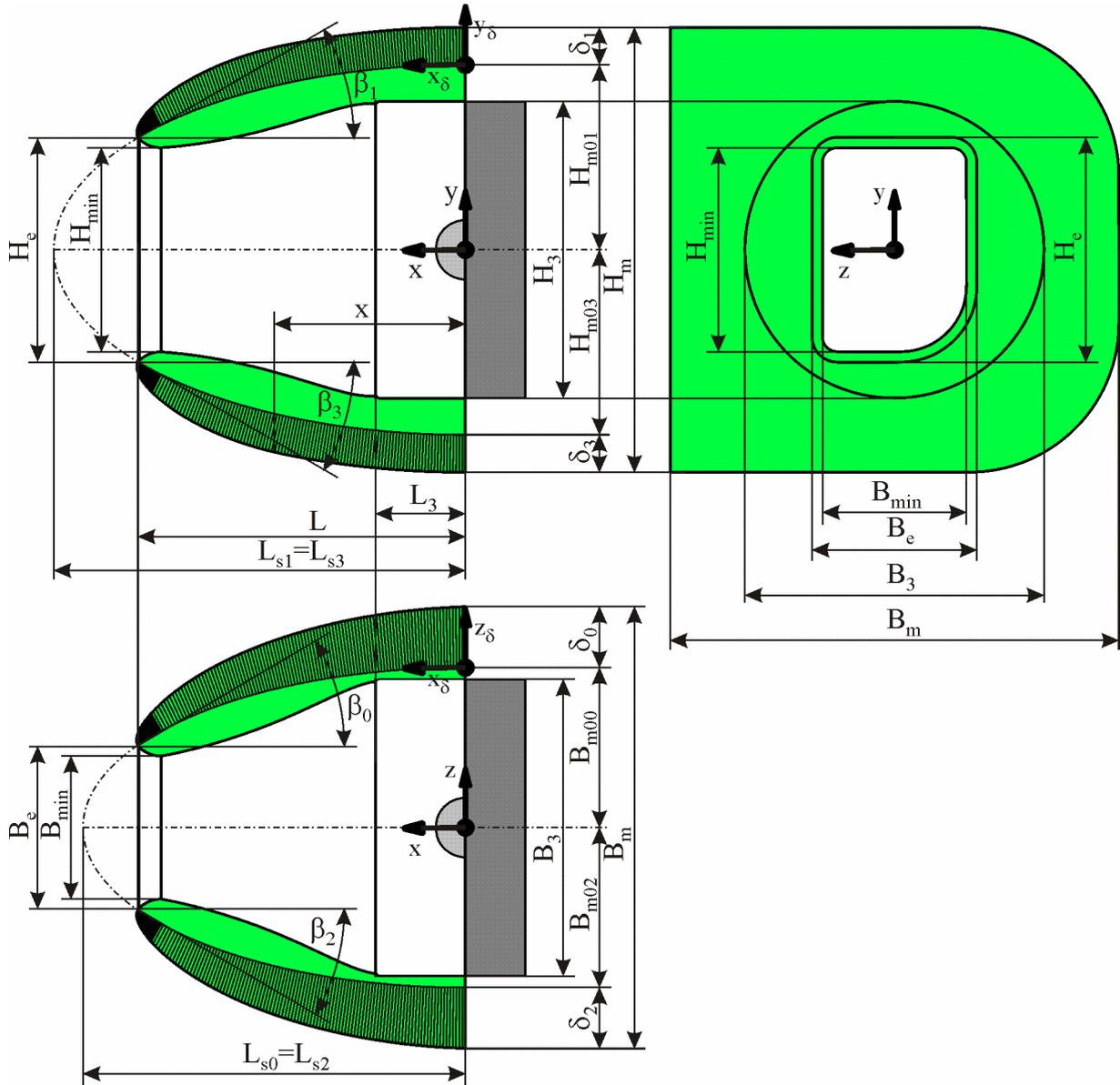
Fig. 3. Design model of non-circular air intake
