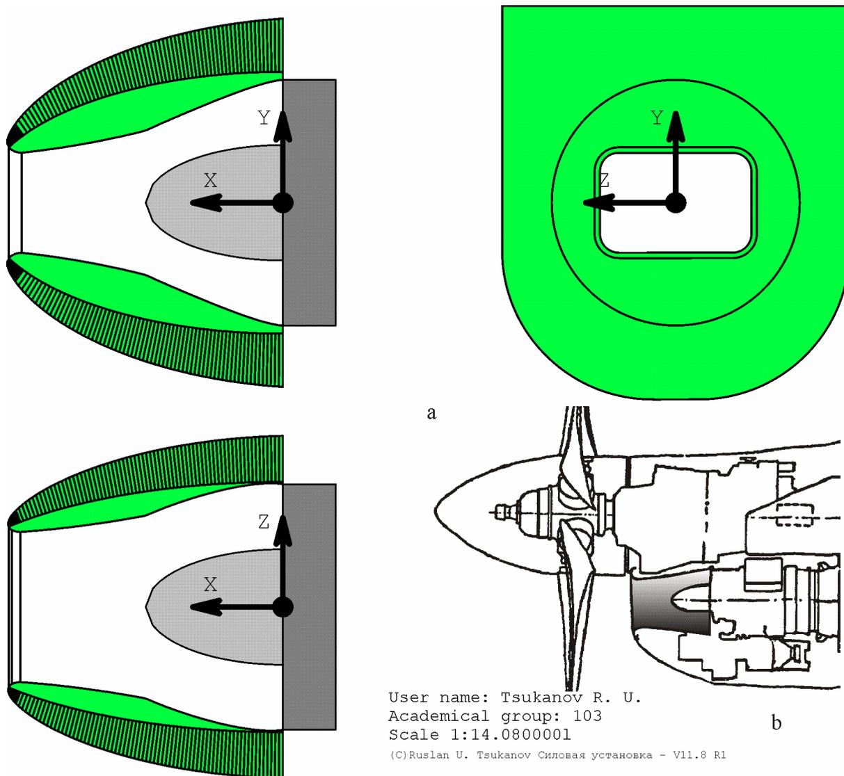
Fig. 5. Air intake of TB3-117BMA-CBM1 engine:
