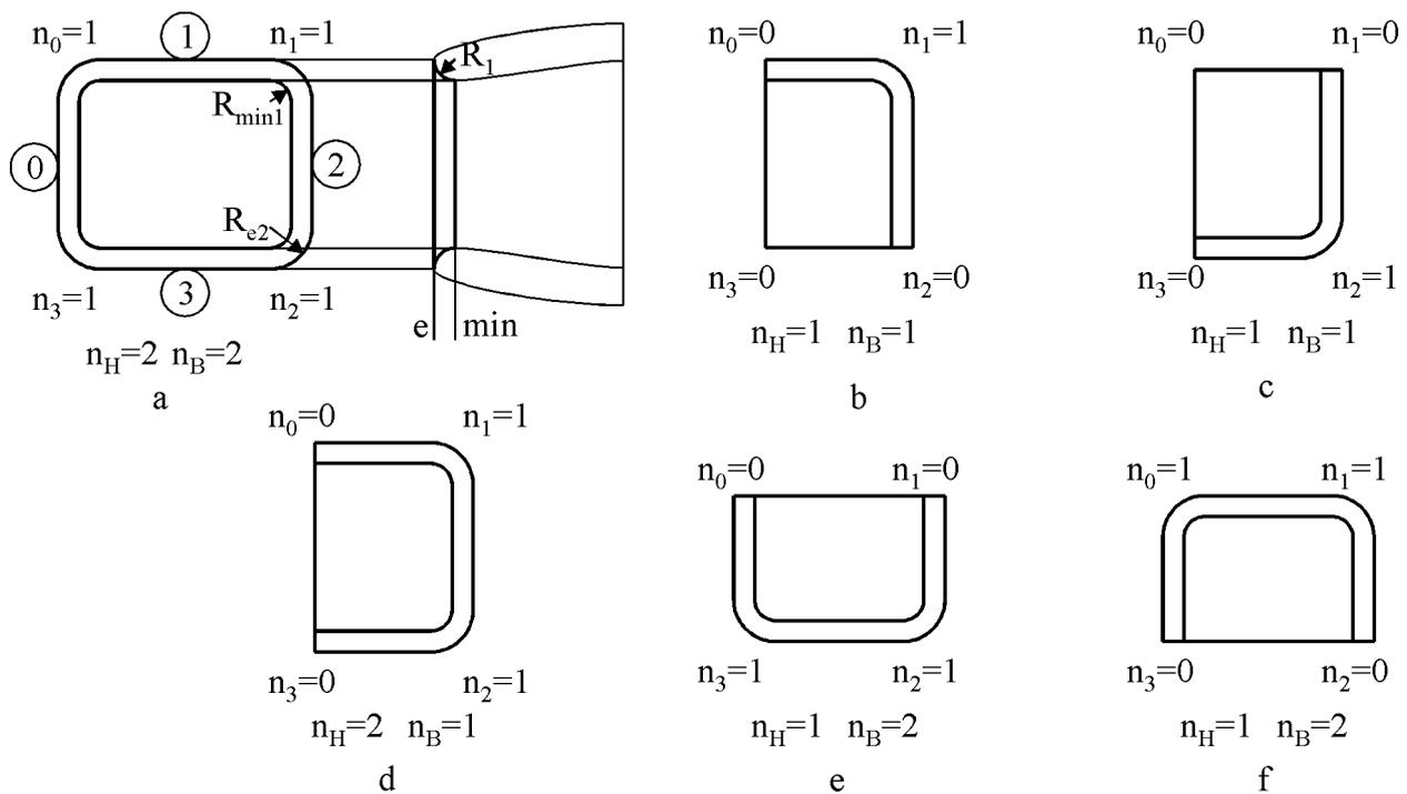
Fig. 2. Determining parameters of minimal and inlet cross-sections
