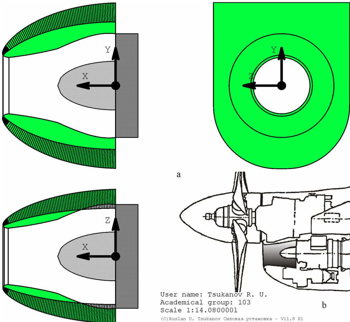
Fig. 4. Air intake of TB3-117BMA-CBM1 engine:
