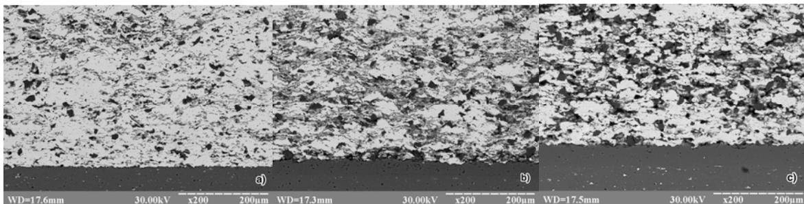
Figure 2 - SEM images at the 200x Amplification for specimens sprayed at 424 C (a), 526 C (b) and 632 C (c). In the microstructure the black particles are non-deformed Alumina particles that were impregnated into the coating
