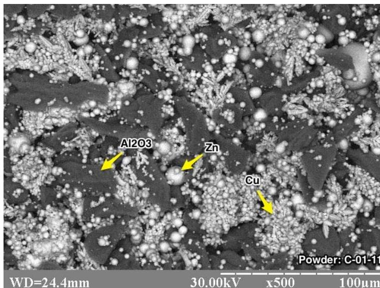
Figure 1 - Morphology of powder C-01-11 Powder in a blend of 65%wt.%Cu+10wt.%Al<sub>2</sub>O<sub>3</sub>+25wt.%Zn provided by OCPS
