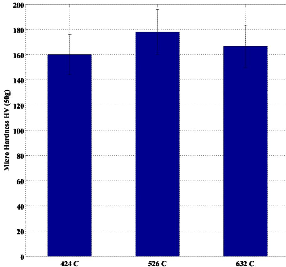
Figure 4 – Results of micro-hardness readings
