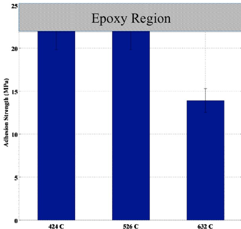
Figure 3 – Adhesion test results for C-01-11 coatings sprayed at different stagnation temperatures
