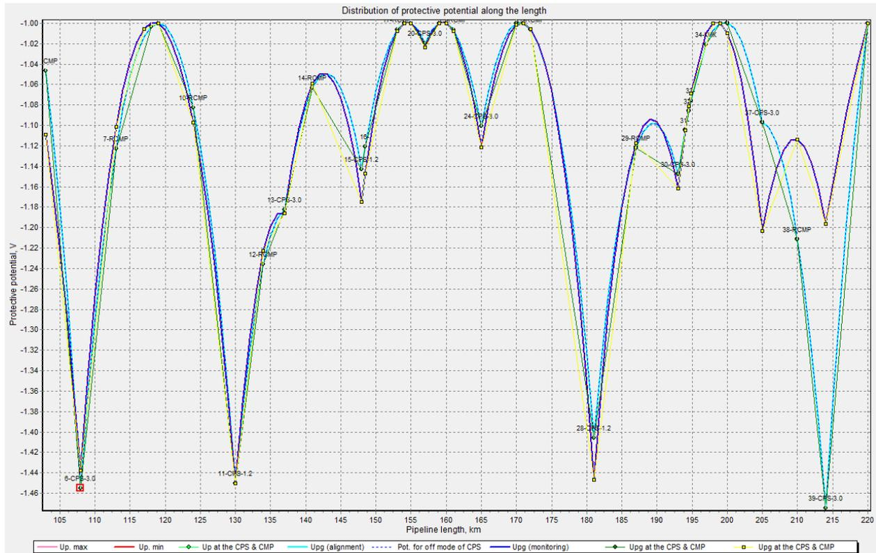
Fig. 5. A new plan for the distribution of the total potential, adjusted from top to  $U_{PGjmin}$  and from bottom to  $U_{PGjmax}$
