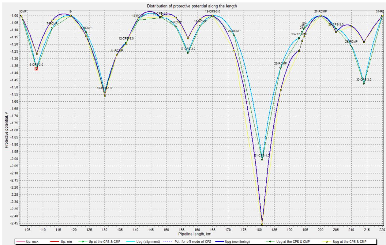
Fig. 7. The new plan for the disconnected CPS for 165 km of pipeline
