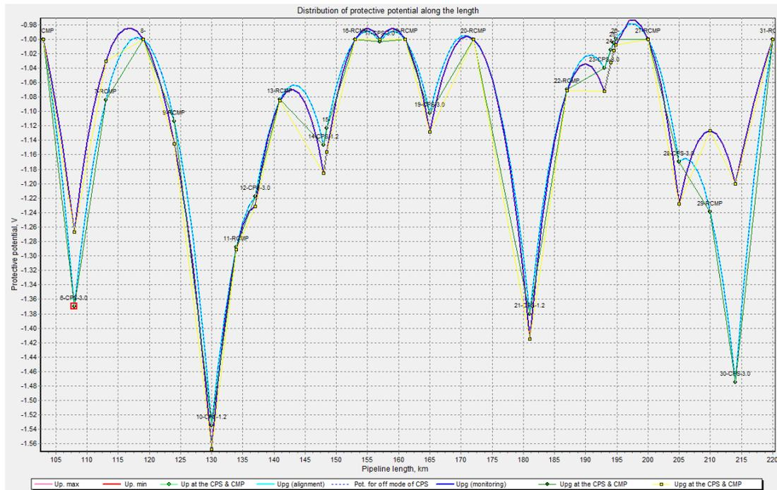
Fig. 4. The initial plan after minimizing the total current of all CPS on the site
