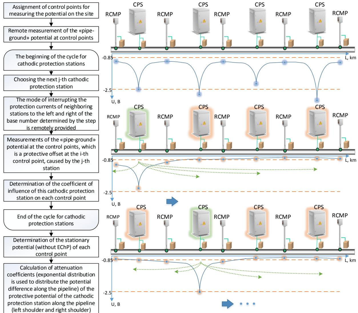
Fig. 1. The scheme of the adjustment technique for finding the effect of CPS
