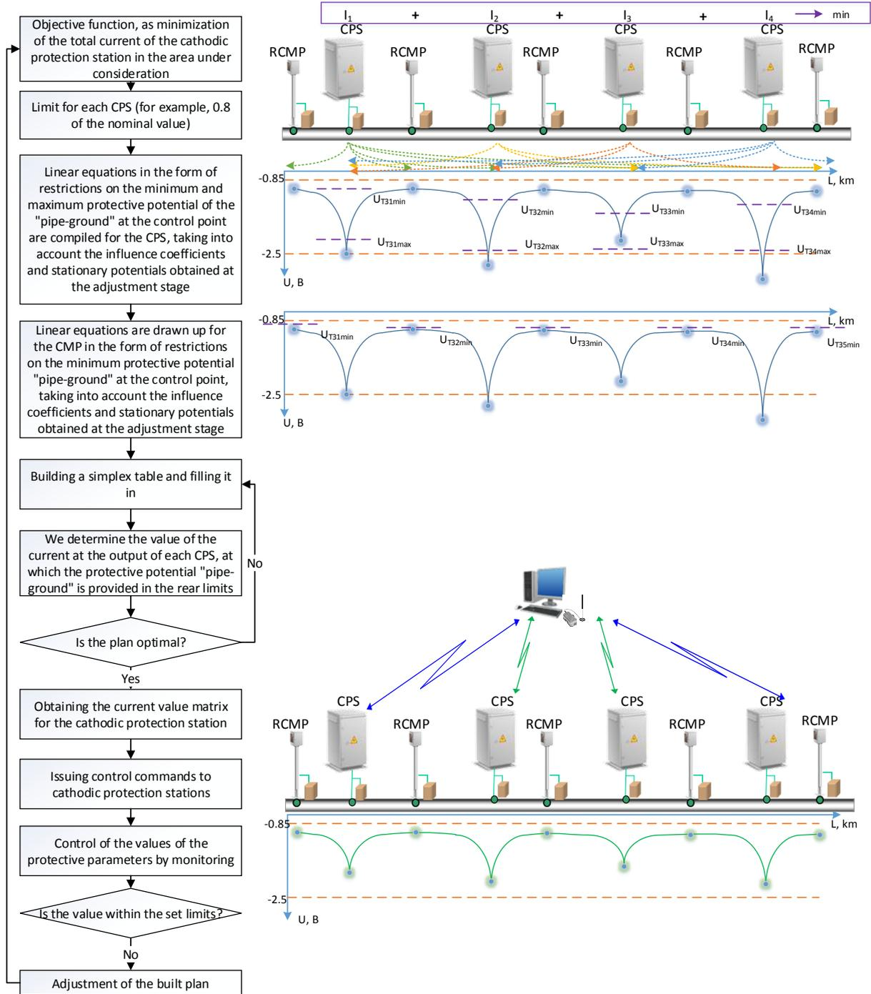
Fig. 2. Scheme of the methodology for optimizing the protective parameters of the CPS
