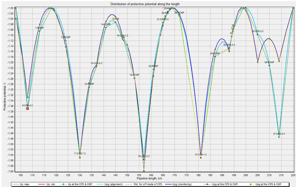
Fig. 8. A new plan for the distribution of the total potential, with the CPS disconnected for 165 km of pipeline, adjusted from above to  $U_{PGjmin}$  and from below to  $U_{PGjmax}$
