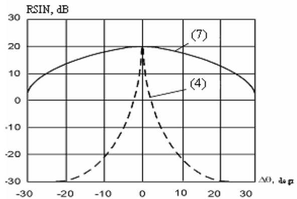
Fig. 3. Dependence of output RSIN on the value of error in the direction of signal arriving
