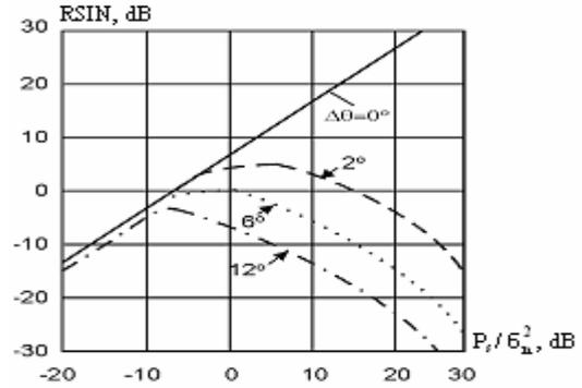
Fig. 1. Dependence of output RSIN on the input relation signal/noise
