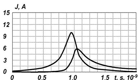
Fig. 5. Dependencies of the discharge current (upper curve) and plasma electron current (lower curve)
