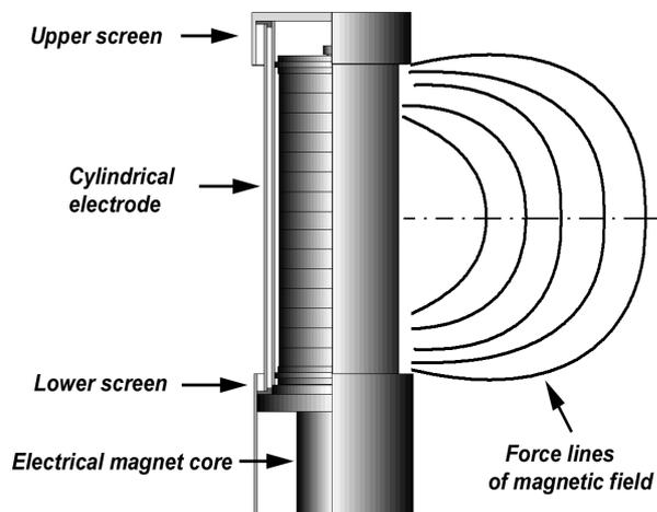
Fig. 2. Scheme of the cylindrical probe
