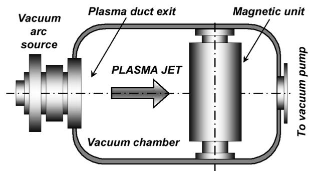
Fig. 1. Scheme of the experiment with cylindrical probe
