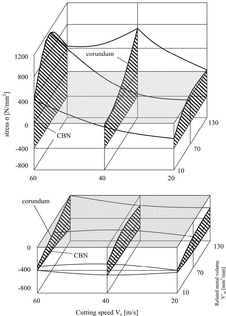
Fig. 3. Effects of oil as a grinding fluid
