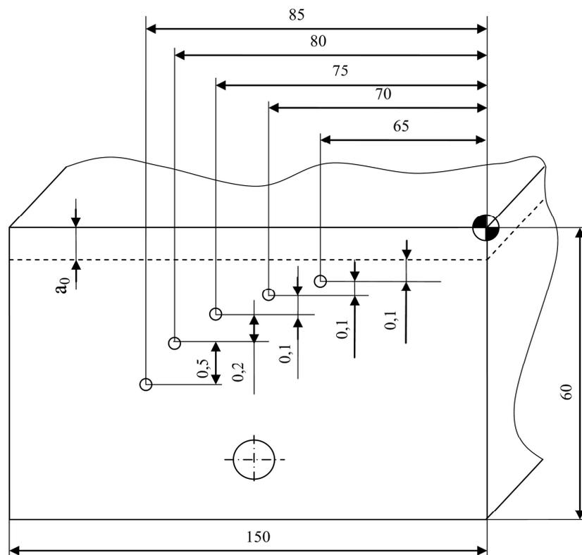
Fig. 4. Schematic of thermocouple technique for measurement of surface temperatures during grinding
