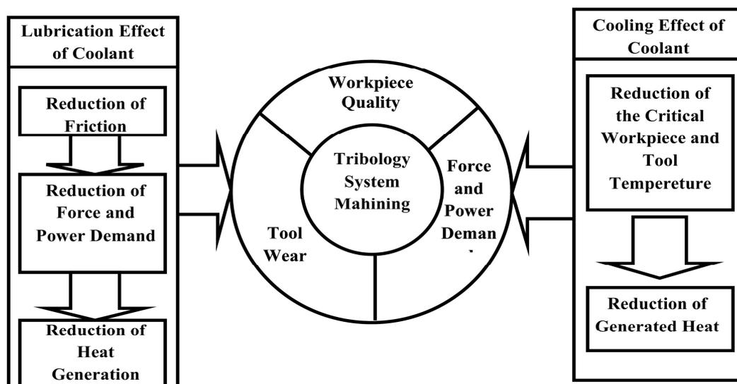
Fig. 1. Primary effects of lubrication and cooling in the machining process after Brinksmeier et al. (1999)
