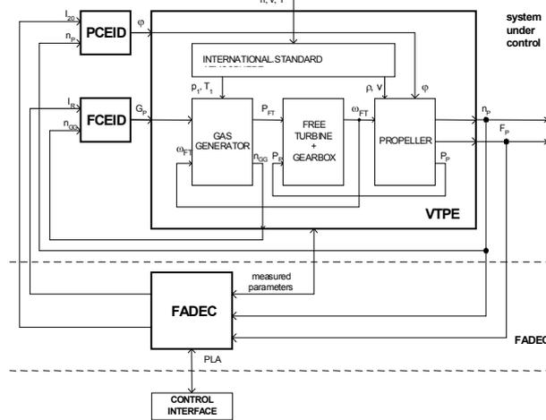
Fig. 4. Block diagram of the VTPE and CP-CS architecture
