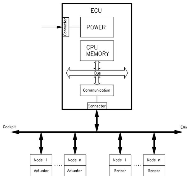
Fig. 1. Distributed control system architecture
