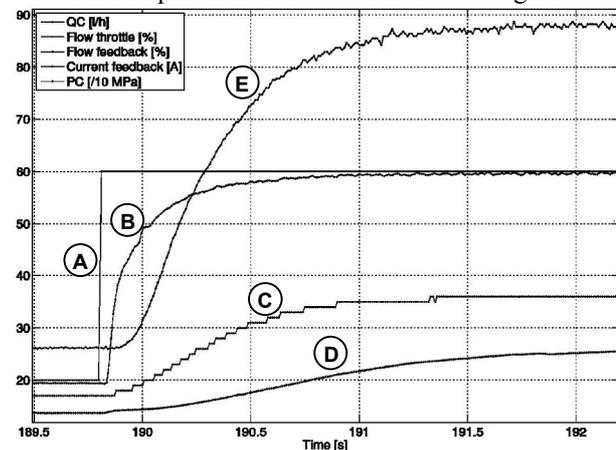
Fig. 9. FMP starting sequence measured on the fuel circuit simulator
