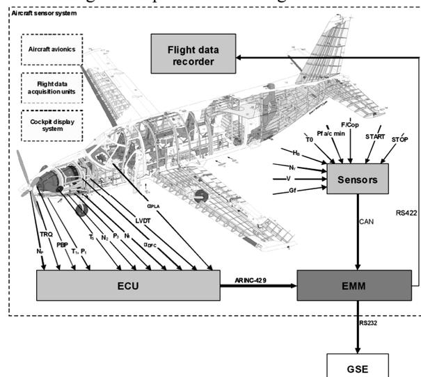
Fig. 3. Design concept of engine monitoring system
