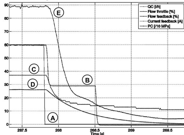
Fig. 10. FMP stopping sequence measured on the fuel circuit simulator
