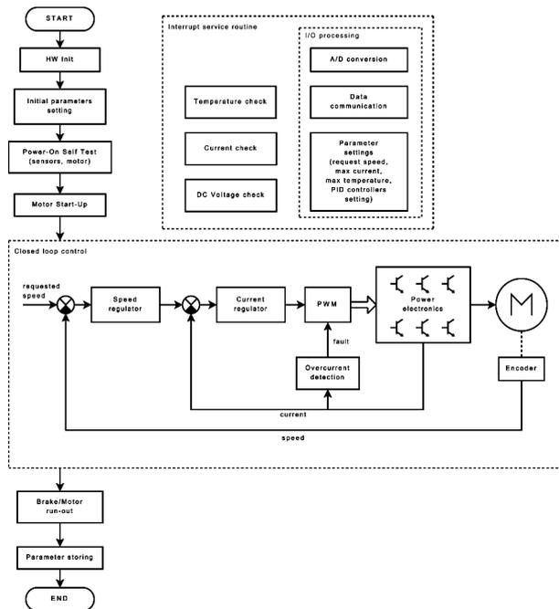
Fig. 8. Concept of the control system software design
