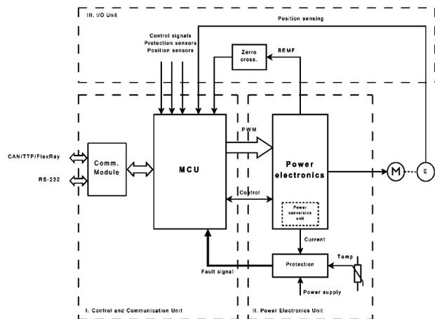
Fig. 6. Architecture of the electronic control system for EHA/EMA actuators
